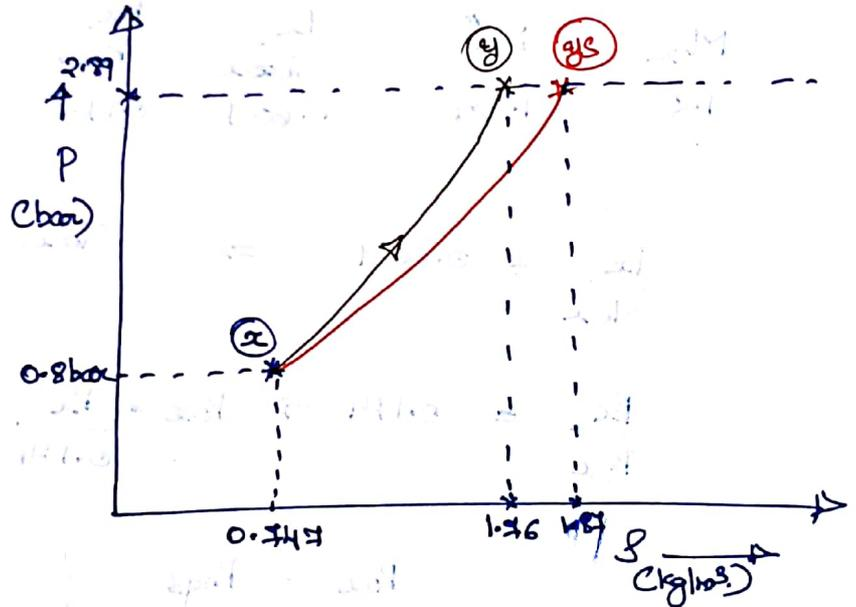
Note: We see that through isentropic compression for given pressure ratio exit Mach number is 0.84 which is subsonic. Hence supersonic diffuser in this case should be a C-D duct to decelerate flow from supersonic to subsonic.
