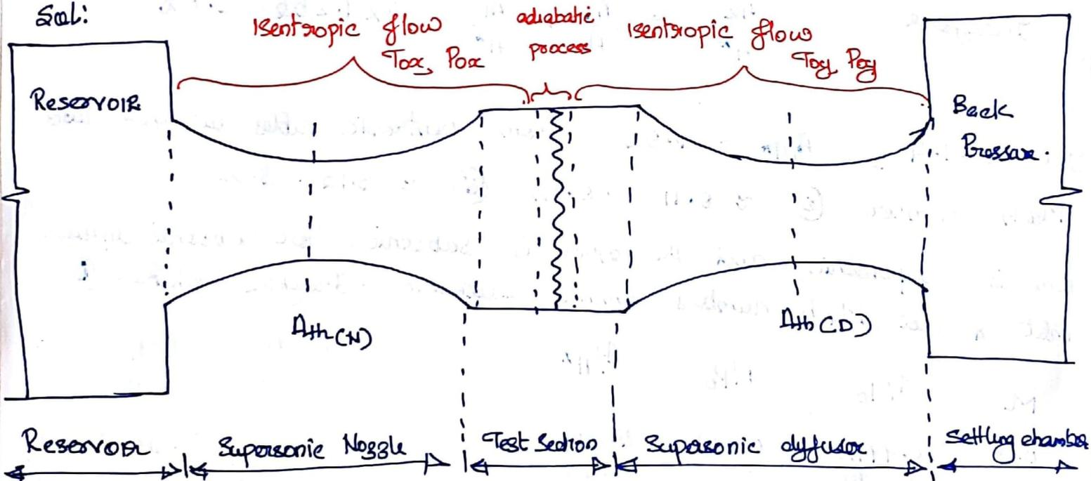
A supersonic wind tunnel aims at generating supersonic flow in the test section. For this air from reservoir is accelerated using supersonic nozzle. Test are conducted with supersonic flow at test section. After this low pressure high velocity fluid is compressed through a supersonic diffuser and raised to ambient & expelled out. To maintain this flow the back pressure is lowered using vacuum pump.
