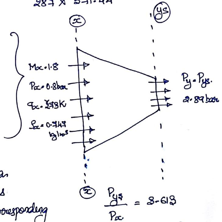
When the supersonic flow encounters a normal shock the Mach number reduces from '1.8' to '0.618'. There is a corresponding increase in pressure down stream of shock (shock is a compression wave). From calculation it was found that pressure increases from " $P_x = 0.8 \text{ bar}$ " to " $P_y = 2.89 \text{ bar}$ " when the fluid passes through normal shock. Hence pressure ratio  $\frac{P_y}{P_x} = 3.613$ .
